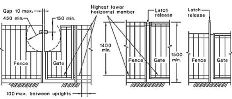
(c) Shield larger than minimum size (d) Shield not required for latch or release located at 1500 or higher
